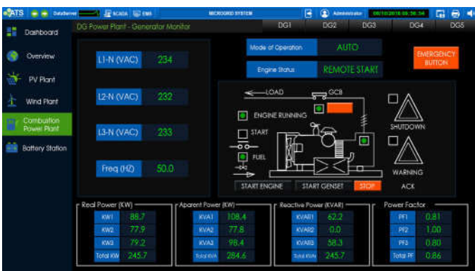
Figure 10. Specific Diesel Generator Monitoring
