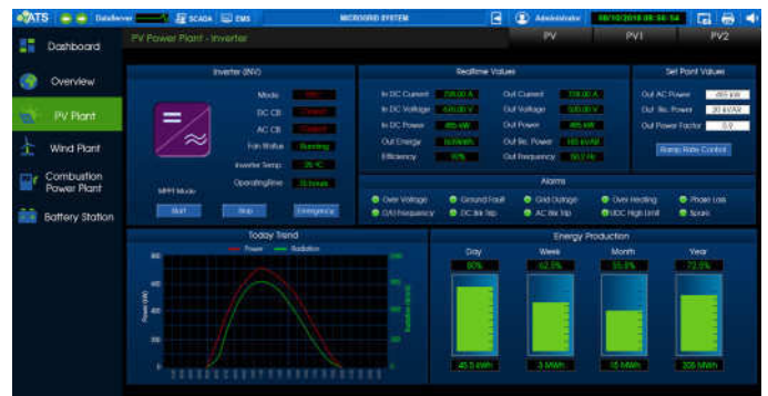
Figure 8. Specific Inverter Unit Monitoring
